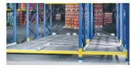
To avoid damage in everyday use, entry guides and roller protectors are an extremely robust design
